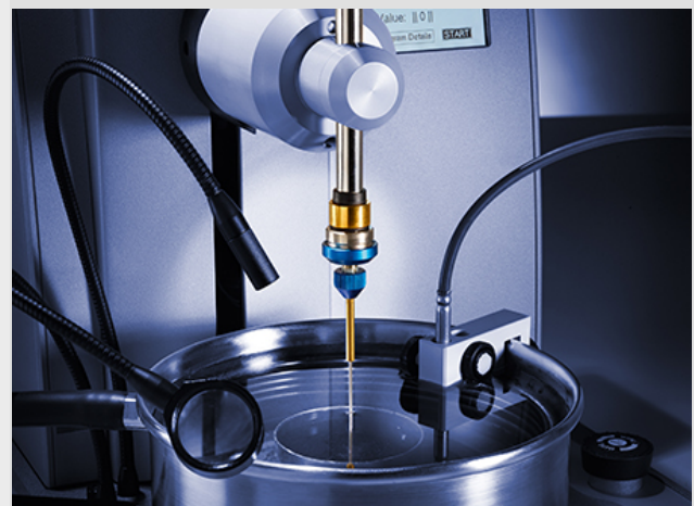
Fig. 1 Automatic surface detection under water
